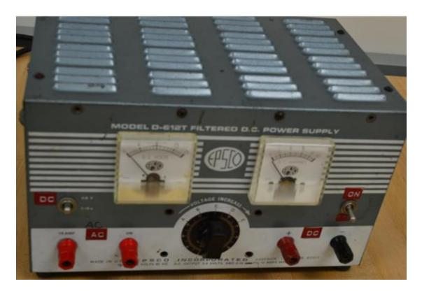
Pictured above are the elderly variacs used in the lab. We had them from years ago and used them again as needed. Pictured below are the dc power supplies used. We needed at least 6 A of 12 V power to run some of the motor experiments and these were the only ones capable of 6 or higher Amps.
