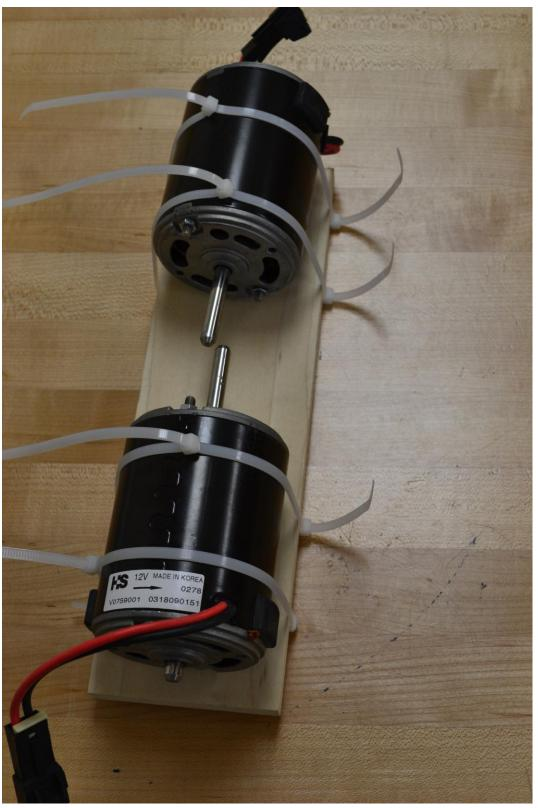
Pictured here are the two motors mounted to a board. The boards were bought from Home Depot and used for mounting of equipment. Here can be seen the need for coupling between the motors. We used surgical tubing and duct tape. The combination worked quite well.
